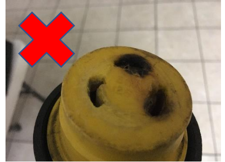
Figure 2 - Burnt connectors - Jim Philip
